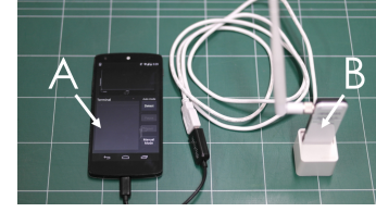
Figure 5: A prototype of PrAP-Hunter. (A) PrAP-Hunter, (B) channel interference device
