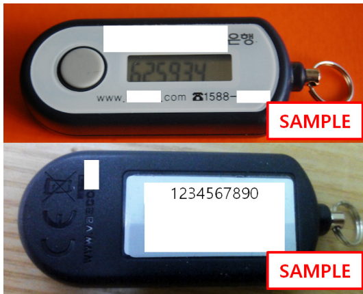
Fig. 3. The OTP generator used in online banking
